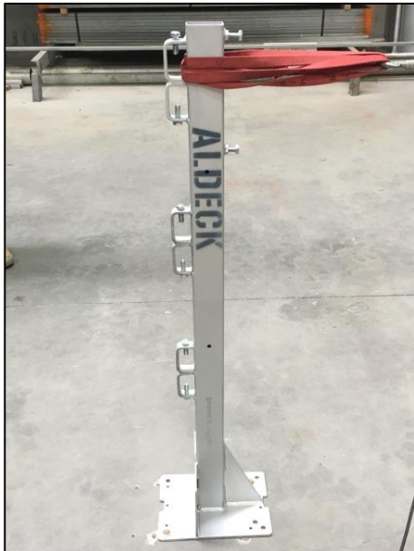
Figure 1: 1100mm temporary guardrail post
